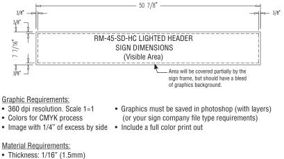
• Good- Acrylic/Pexiglass, Better - high impact acrysteel, acrylite SG Best- Super impact Lexan, Lexan SG Polycarbonate
